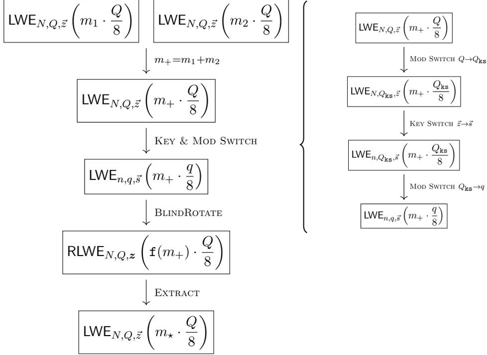
Figure 3: Steps modification bootstrapping for NAND gate [CGGI20, LMK<sup>+</sup>23]
