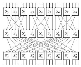
layers. Examples for (m, t) = (4, 2) and (3, 3) are shown in Figure 1.7. However, there is a problem with their construction: it can be shown that if a single input bit is changed, the probability of an output bit changing will always be  $2^{-t}$ . This was shown in [Web85] and termed avalanche damping (see also [WT85]).
