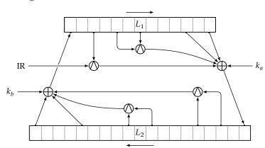
Figure 3.37: The Structure of KATAN/KTANTAN
