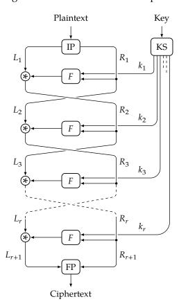
Figure 1.3: Schema of a Feistel Cipher
