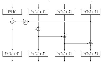
Figure 3.26: The AES Key Schedule for 128-bit Keys
