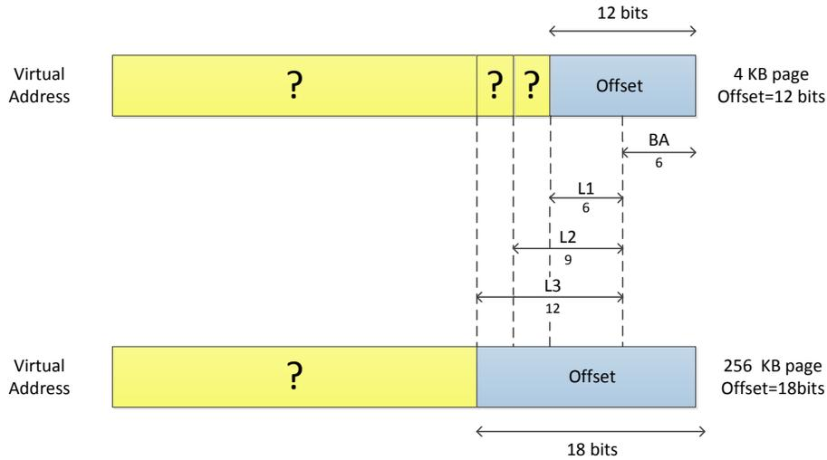
**Fig. 2.** Regular Page (4 KB, top) and Huge Page (256 KB, bottom) virtual to physical address mapping for an Intel x86 processor. For Huge pages the entire L3 cache sets become transparently accessible even with virtual addressing.
