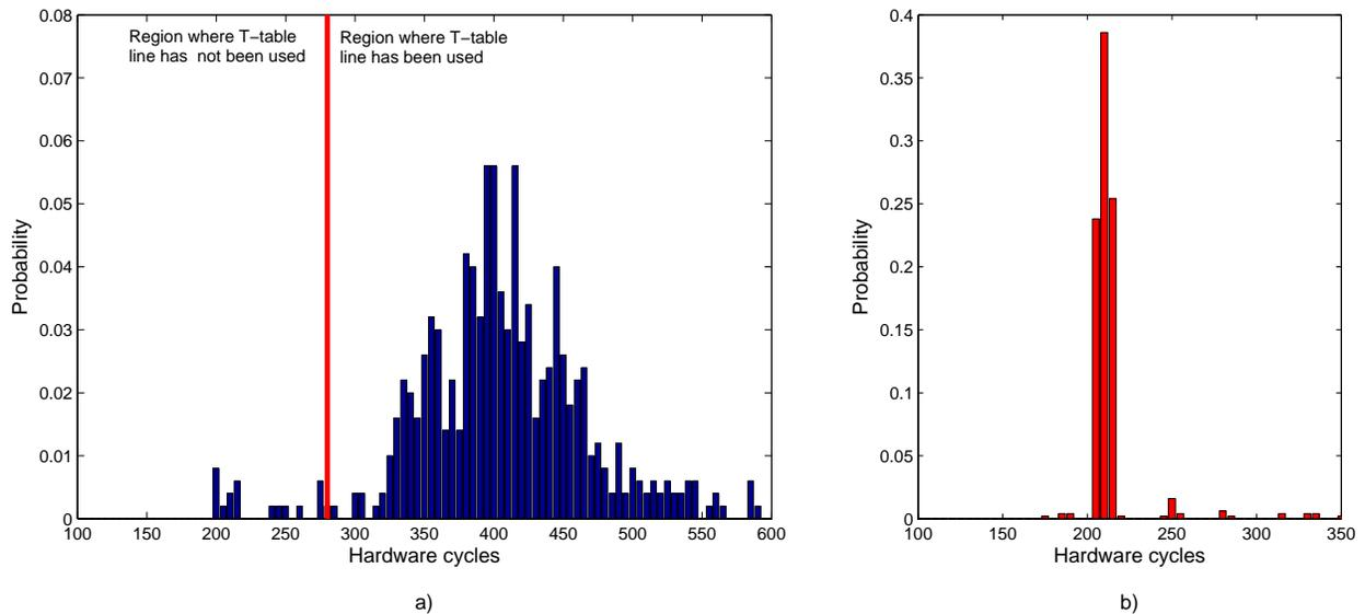
**Fig. 5.** Histograms of 500 access times monitored in the probe stage for a) a set used by a T-table memory line and b) a set not used by a T-table memory line. Measurements are taken in the Xen 4.1 cross-VM scenario.
