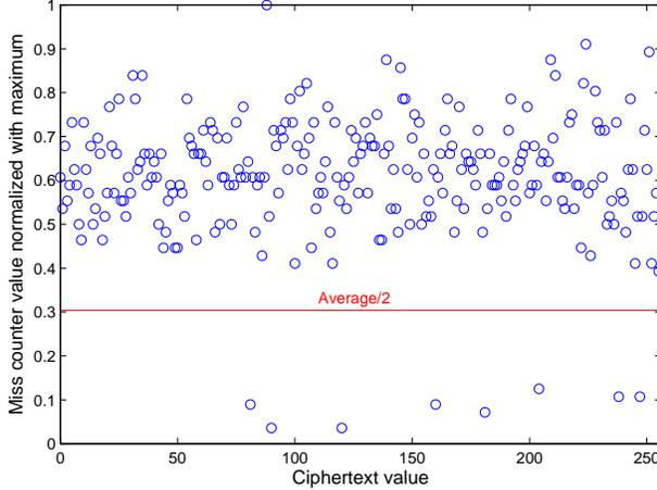
**Fig. 6.** Miss counter values for ciphertext 0 normalized to the maximum value. The key is e1 and we are monitoring the last 8 values of the T-table (since the table starts in the middle of a memory line).
