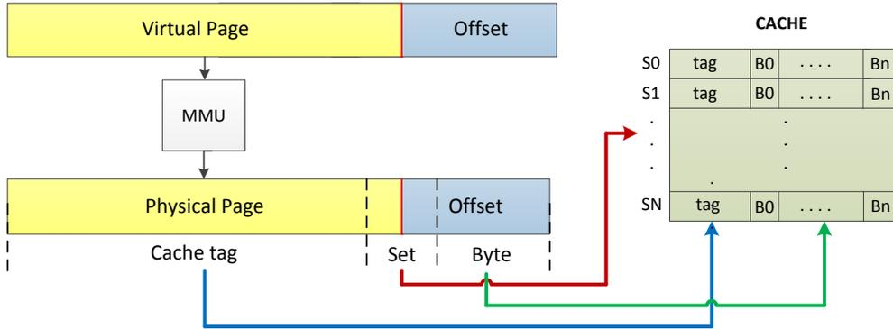
**Fig. 1.** Cache accesses when it is physically addressed.
